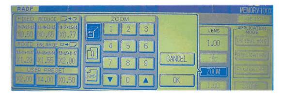
Key in the desired zoom ratio. It will be displayed under "Lens Mode ". Press "OK" when you have obtained your desired zoom ratio.
